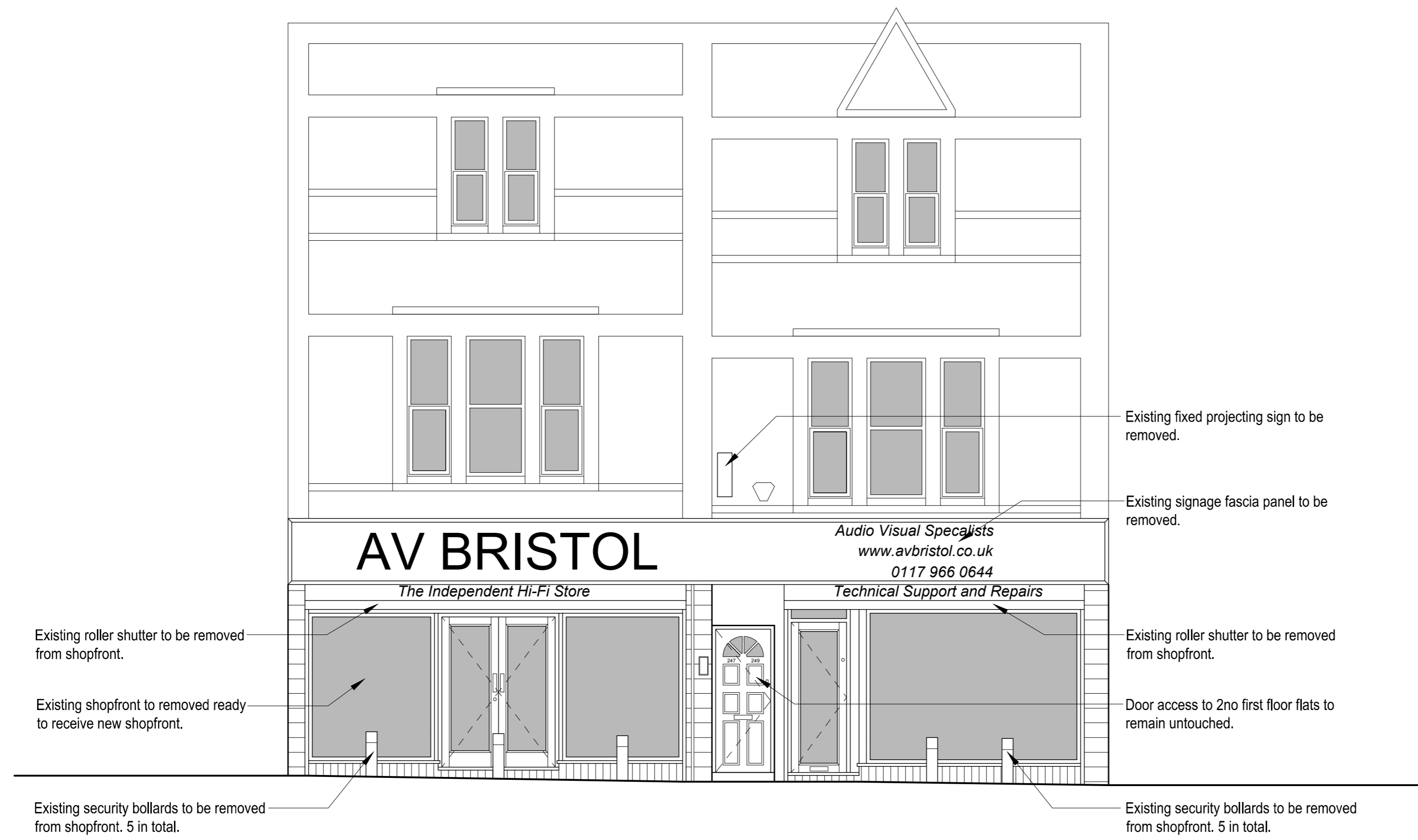
EXISTING FRONT ELEVATION
